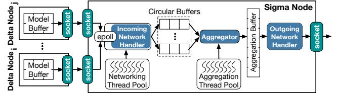
Figure 2: System software in a Sigma node.
