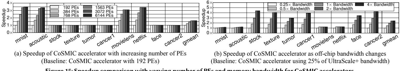
Figure 15: Speedup comparison with varying number of PEs and memory bandwidth for CoSMIC accelerators.
