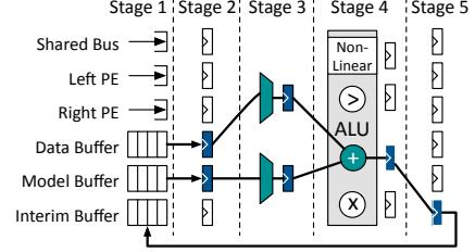
Figure 6: Pipelined PE. Black highlights an Add operation ( $\text{Interim-Buffer}[i] = \text{DataBuffer}[j] + \text{ModelBuffer}[k]$ ).
