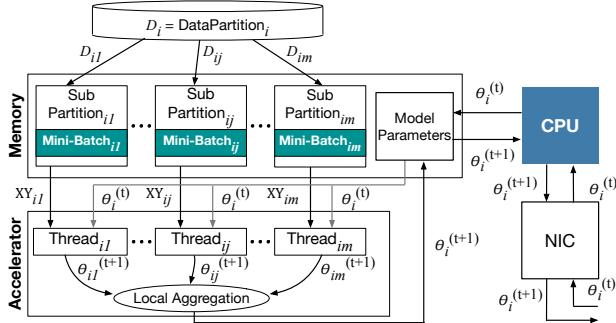
Figure 1: Execution and acceleration flow within each node.
